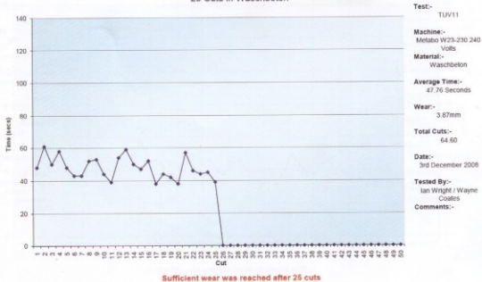
Graph to show Tyrolit Universal Fast Cut Basic Ø230mm x 8mm Segment Cutting Times 25 Cuts in Waschbeton
