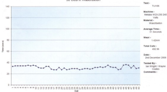
Graph to show Mi750 Marcrisr New No WC Ø230mm x 10mm Segment Cutting Times 50 Cuts in Waschbeton
