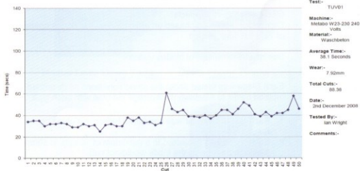
Graph to show Dieve Master Drive Universal Ø230mm x 10mm Segment Cutting Times 50 Cuts in Waschbeton
