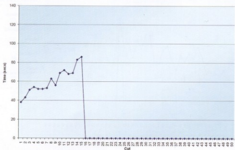
Graph to show Spectrum Cyclone ZCX Ø230mm x 10mm Segment Cutting Times 15 Cuts in Waschbeton
