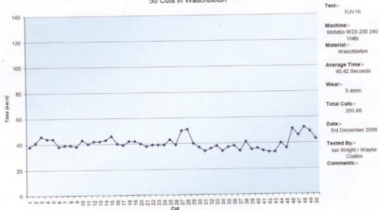
Graph to show Rothermberger Red Professional Ø230mm x 10mm Segment Cutting Times 50 Cuts in Waschbeton
