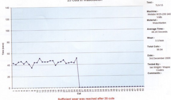
Graph to show Norton Clipper Classic Jet Ø230mm x 10mm Segment Cutting Times 25 Cuts in Waschbeton
