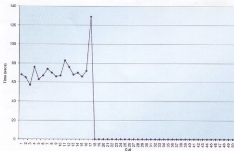
Graph to show Edge Sintered Sitemaster Trade Segmented Ø230mm x 10mm Segment Cutting Times 17 Cuts in Waschbeton
